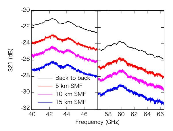
Frequency response of RoF link at 40-48 GHz and 56-67 GHz bands
