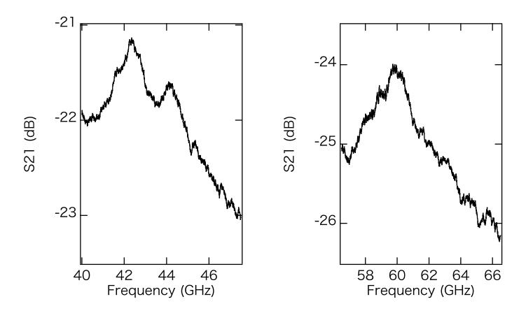
Amplitude Deviation: < 2 dBp-p at 40.5-47 GHz ~ 2 dBp-p at 57-66 GHz
