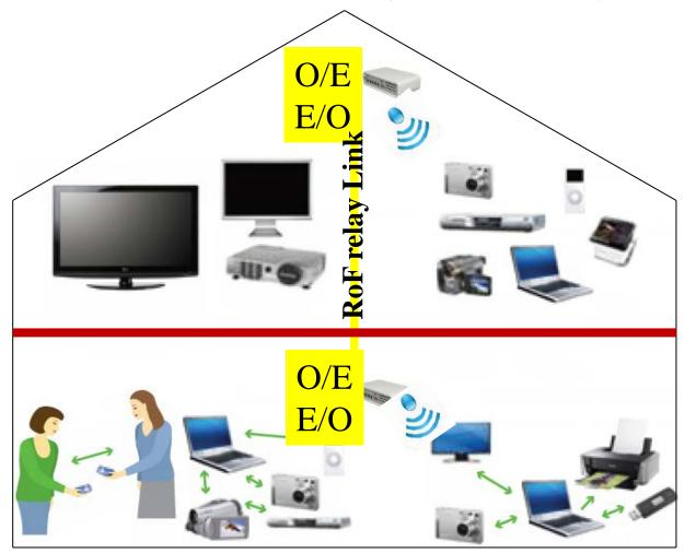
45 GHz and 60 GHz frequencies cannot penetrate walls, floors and ceilings in the buildings.
